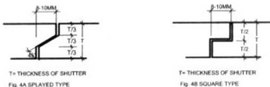
Fig. 4 : Meeting of Stiles for Double Leaved Shutters
